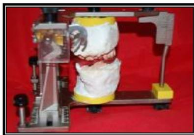
**Figure 7 a: Estimation of the protrusive angle.**
