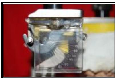
**Figure 6: The condyle pin located at the protractor center.**
