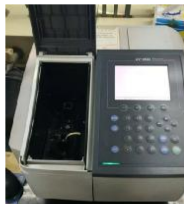
Figure 2: The Sample in the Spectrophotometer (uv-1800 SHIMADZU / Japan)
