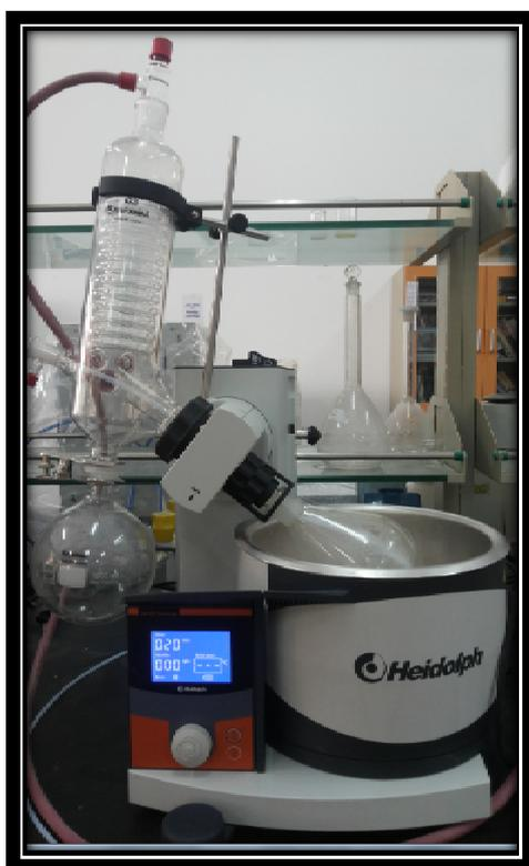
**Fig.2: Rotary evaporator**
