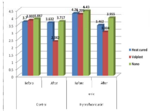
**Figure 8: Bar chart of the mean value of shear bond strength in (MPa) for all types of denture bases bonded to porcelain teeth before and after thermocycling.**
