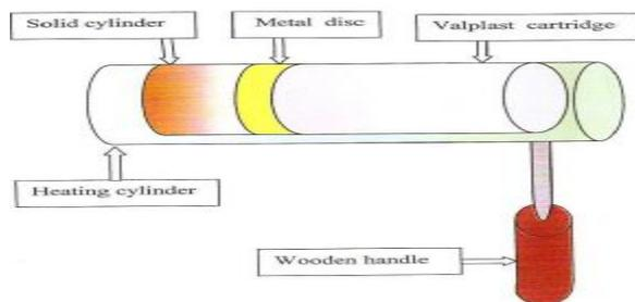
**Figure 5: the configuration of the injection system.**
