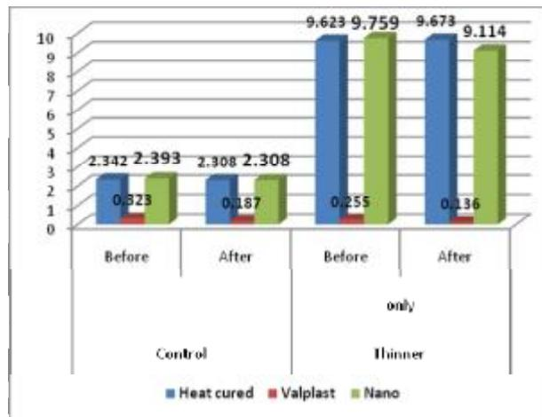
**Figure 7: Bar chart of the mean value of shear bond strength in (MPa) for all types of denture bases bonded to acrylic teeth before and after thermocycling.**
