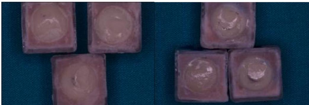
Figure 3: Cohesive failure within ceramic. Figure 4: Combination failure (adhesive/cohesive).
