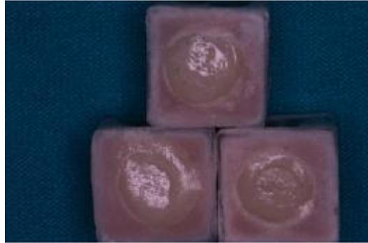
**Figure 5. Adhesive failure**
