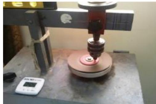
Figure 3: Wear rate testing machine
