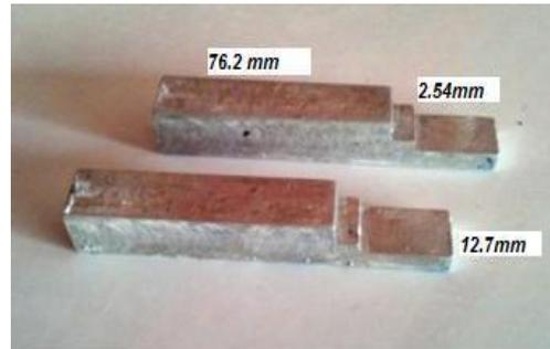
Figure 2: Metal pattern for shear bond test
