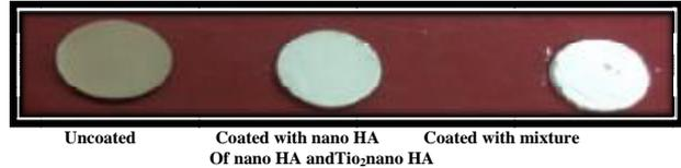
Figure 3: Coated CP Ti discs for in vitro study
