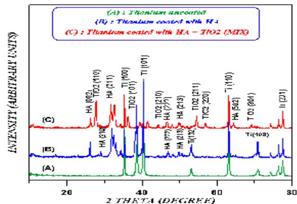
Figure 9:X-ray diffraction patterns of nano HA and mix of nano Tio<sub>2</sub> and nanoHA coated CPTi specimen in comparison with the uncoated specimen.
