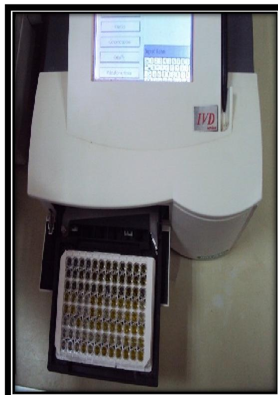
**Figure 10: Microplate ELIZA reader device**
