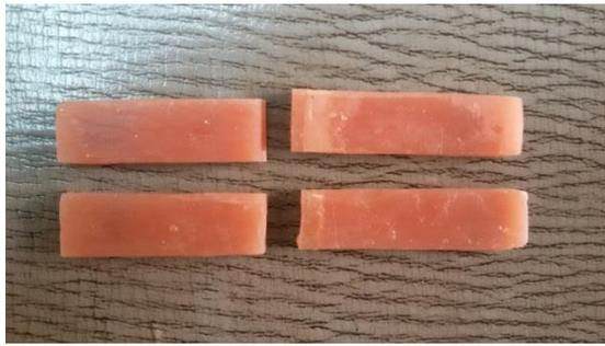
Figure 4: Repaired samples after finishing the transverse strength testing.
