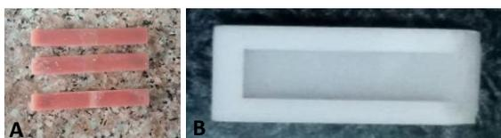
Figure 2: (A): Repaired samples ready for testing; (B): Plastic orientation device for sample holding.
