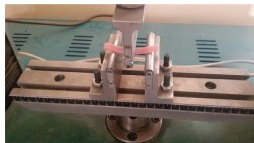
Figure 3: Instron universal testing machine during sample testing.
