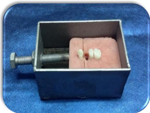
**Figure 1: Template for teeth fixation.**
