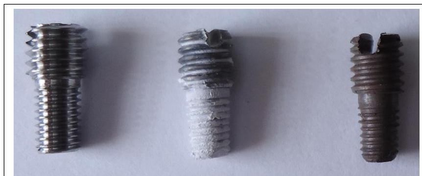
Figure 1: From left: Untreated, Coated with ZrO<sub>2</sub> and Annealed sample.
