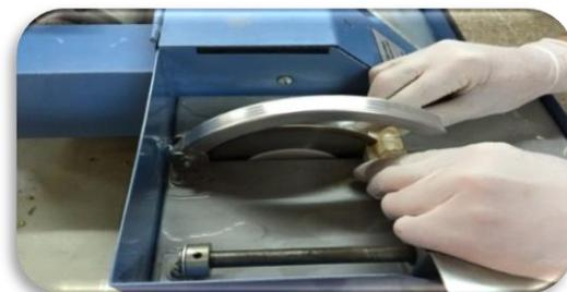
**Figure 4: sectioning machine with water coolant.**
