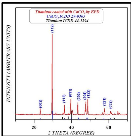
**Figure 2: X-ray diffraction patterns of CaCO<sub>3</sub> coated CP Ti sample using EPD technique**
