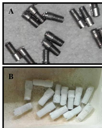
Figure 1: (A) Uncoated implant screws. (B) Coated implant screws with  $\text{CaCO}_3$ . Animal and surgical procedures
