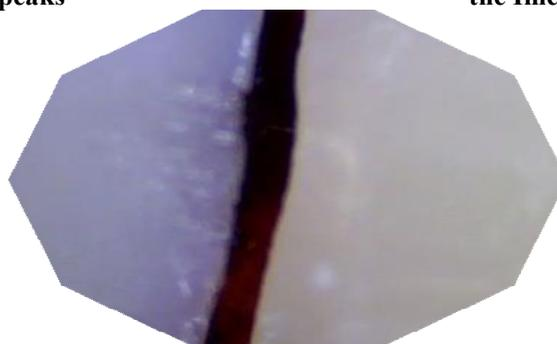
**Figure 14: Enlarged photo of marginal gap of the Dental direct**
