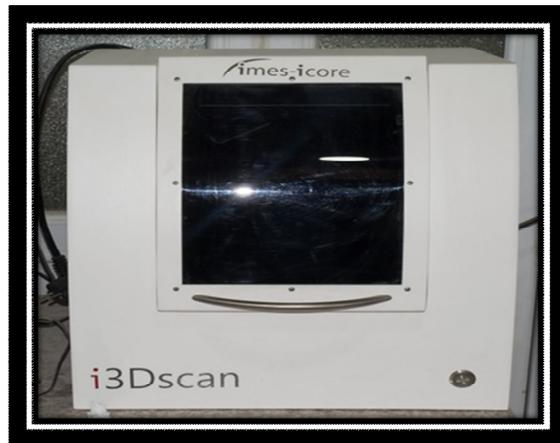
**Figure 4: 3D scan of Imes-icor system.**
