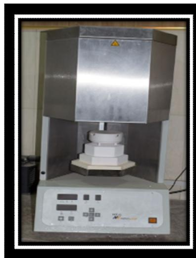
**Figure 7: Sintering oven (HT-S MV mihmvogt-Germany).**
