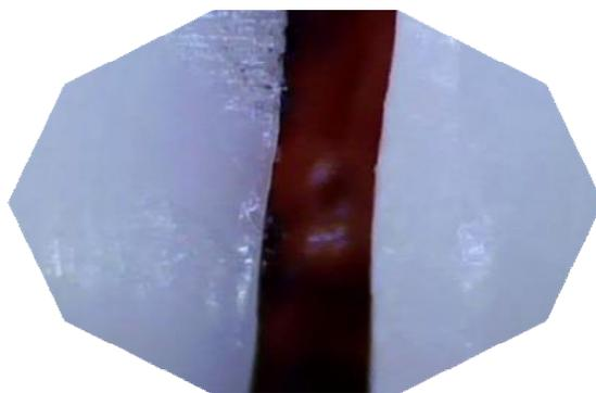
**Figure 12: Enlarged photo of marginal gap of the Whitepeaks**
