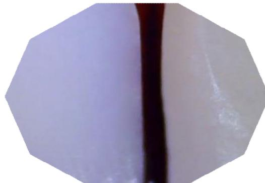
**Figure 13: Enlarged photo of marginal gap of the Imes icor**
