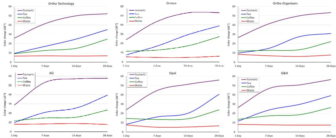
Figure 3: Mean color change of clear elastomeric chains from Ortho Technology, Ormco, Ortho Organizer, AO, Opal and G&H companies after immersion in water, tea, coffee, and turmeric.
