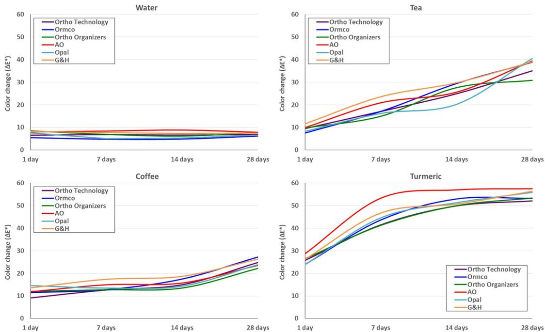
Figure 2: Color changes of elastomeric chains (Ortho Technology, Ormco, Ortho Organizer, AO, Opal and G&H) after immersion in water, tea, coffee, and turmeric.
