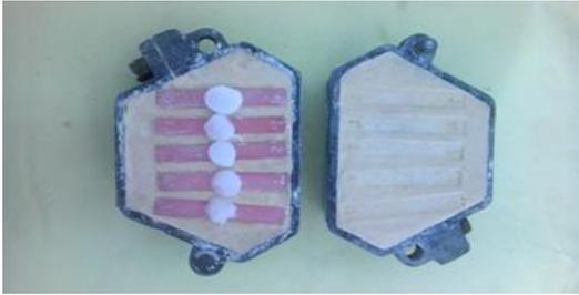
**Figure 2: A fracture nylon specimen placed in the stone mold with 3mm gap for repair material application**
