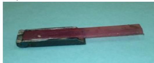
Figure 1: Holding device with 45° bevel joint
