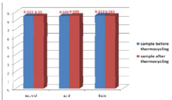
**Figure 5: Bar chart for comparison between means in KJ/m<sup>2</sup> for impact strength samples before and after thermo cycling.**
