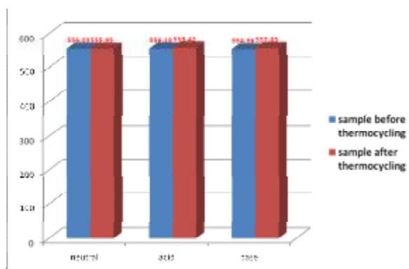
**Figure 8: Bar chart for comparison between means in N/mm<sup>2</sup> for transverse strength samples before and after thermo cycling.**
