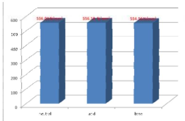
**Figure 6: Bar chart for transverse strength means in N/mm<sup>2</sup> for samples before thermo cycling.**
