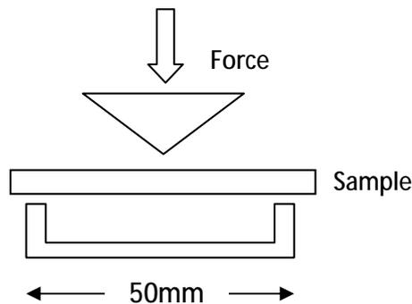
**Figure 2: Schematic illustration of flexural strength test arrangement**
