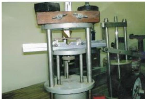
**Figure 3: Flexural testing device**
