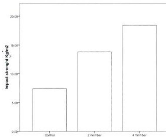
**Figure 5: Graph showing mean impact strength of control and fiber-reinforced PMMA (m=10)**
