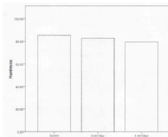
**Figure 7: Graph showing mean hardness of control fiber reinforced PMMA (n=10).**
