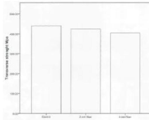
**Figure 6: Graph showing mean flexural strength of control and fiber reinforced PMMA (n=10).**
