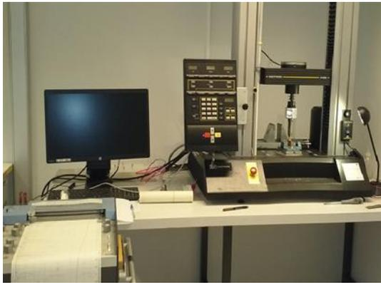
Figure (1) Universal testing machine
