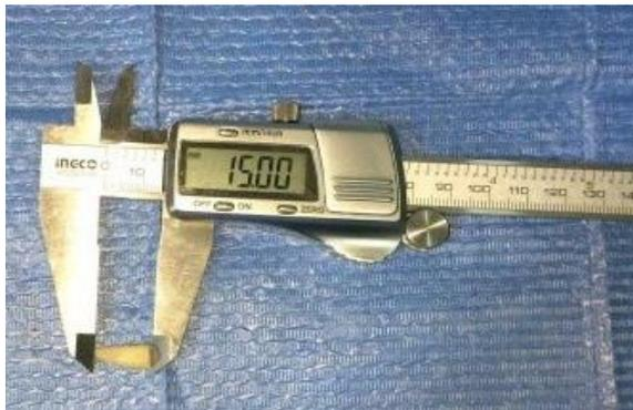
**Figure 1:** Length of tooth was measured with a digital caliper
