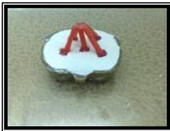
Figure 2. Spruing the wax pattern
