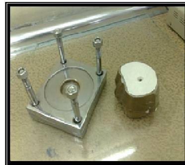
Figure 4. Plastic injection device clamp
