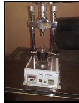
Figure 3. Thermoplastic injection device
