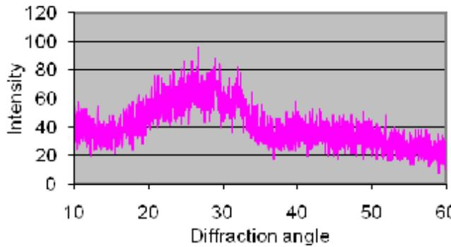
**Figure 7. x-ray diffraction pattern of set glass ionomer cement reinforced by 20% Hydroxyapatite.**
