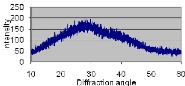
**Figure 3. x-ray diffraction pattern of liquid of glass ionomer cement.**
