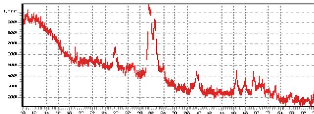
**Figure 1. x-ray diffraction pattern of synthetic Hydroxyapatite.**
