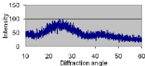
**Figure 2. x-ray diffraction pattern of powder of glass ionomer cement.**
