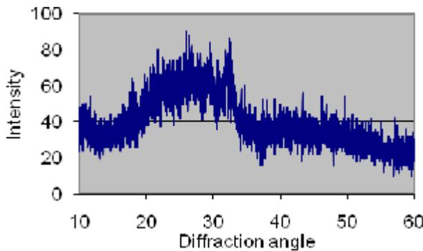
**Figure 8. x-ray diffraction pattern of set glass ionomer cement reinforced by 25% Hydroxyapatite.**
