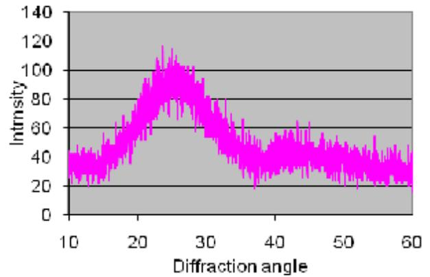
**Figure 4. x-ray diffraction pattern of set glass ionomer cement.**
