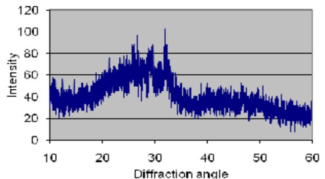
**Figure 6. x-ray diffraction pattern of set glass ionomer cement reinforced by 15% Hydroxyapatite.**
