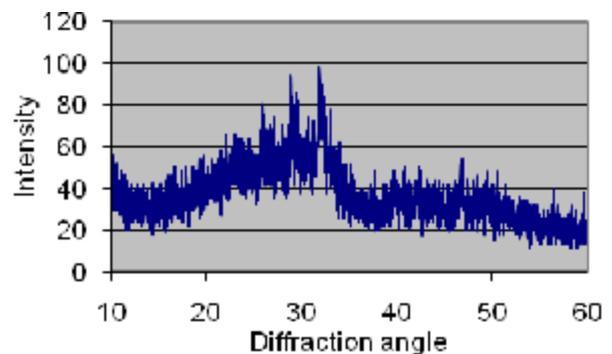
**Figure 5. x-ray diffraction pattern of set glass ionomer cement reinforced by 10% Hydroxyapatite.**
