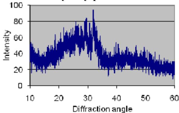
**Figure 9. x-ray diffraction pattern of set glass ionomer cement reinforced by 30% Hydroxyapatite.**
