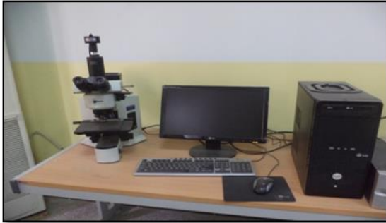
Fig.4: Low lighting microscope used for surface roughness evaluation
