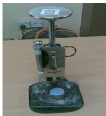
Figure 1: Vicat device for measuring the setting time of gypsum products
