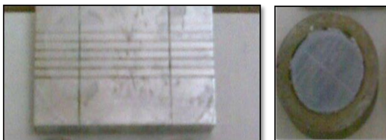
Fig. 2: Metal block for linear expansion test
