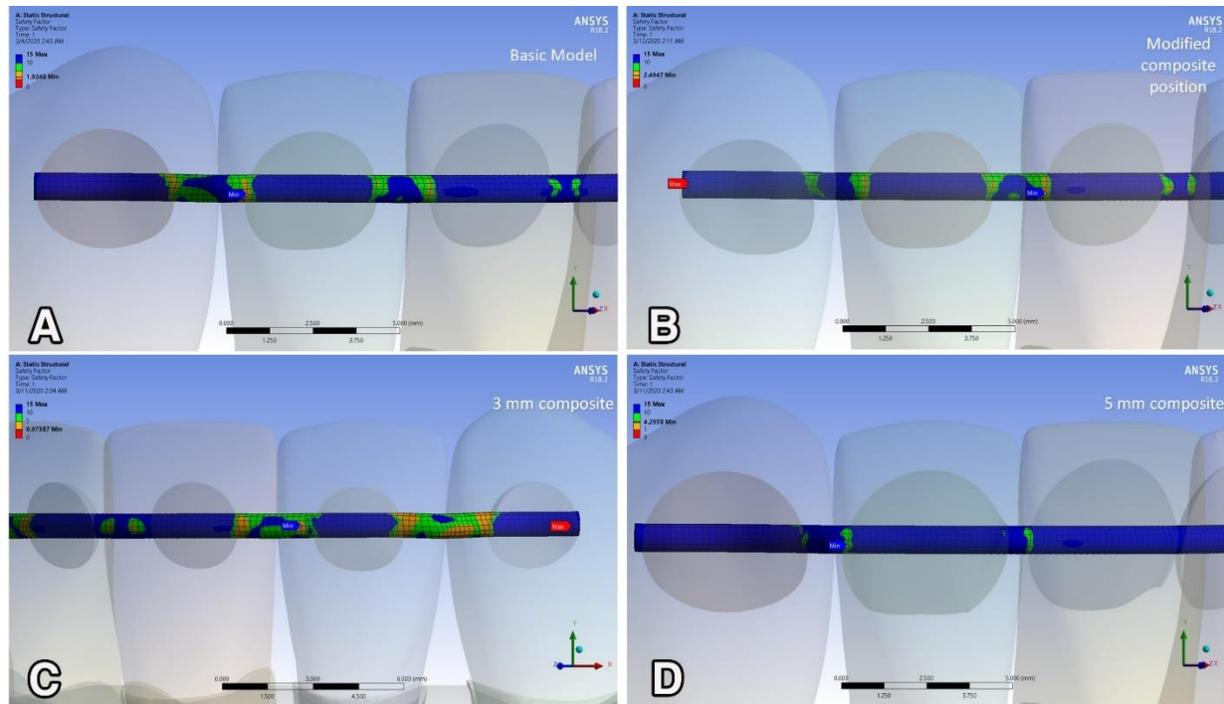
**Figure 5: The safety factor of PEEK in four models, the blue indicator shows the lowest safety factor value i.e., failure site. (A) basic model, (B) modified composite position, (C) 3 mm composite bonding spot, (D) 5 mm composite bonding spot.**
