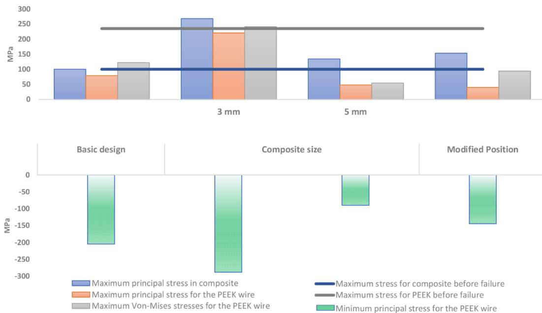
**Figure 4 The effect of the size and position of composite bonding spots on maximum principal stress in composite and PEEK, and maximum von Mises stress in PEEK (Up), and minimum principal stress in PEEK (Down). The blue and grey lines represent the safety limits for composite spots and PEEK wires respectively.**
