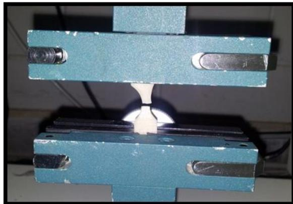
**Figure 5: Testing procedure of Acetal and Co-Cr tensile samples.**
