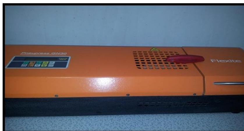
**Figure 3: Acetal flexite injection machine.**
