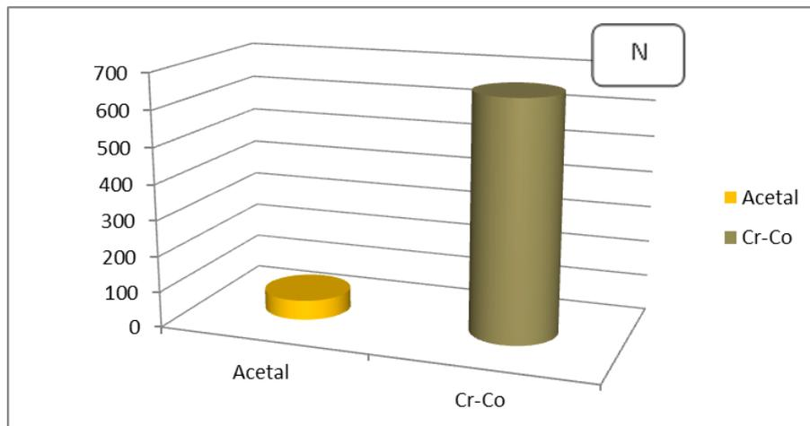
Figure 10: Tensile strength difference between Co-Cr and Acetal.
