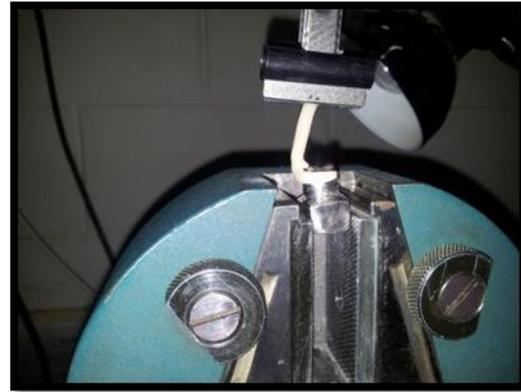
**Figure 4: Testing procedure of Acetal and co-cr clasps,**
