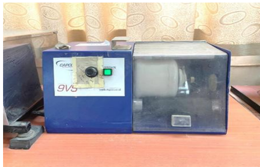
Figure 1: Roller ball mill during operation
