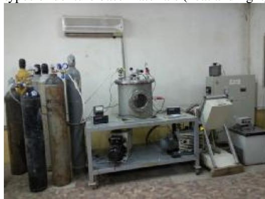
Figure 3: DC-glow discharge plasma device
