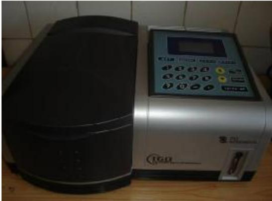
**Figure 2: UV-Visible spectrophotometer (T6UV, KOREA).**
