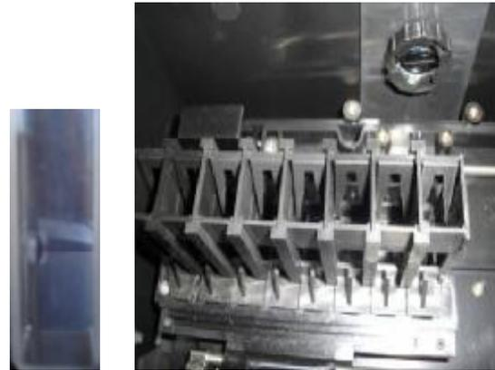
**Figure 3: Black rectangular cardboard with bracket positioned in central window put inside cubit of the spectrophotometer.**
