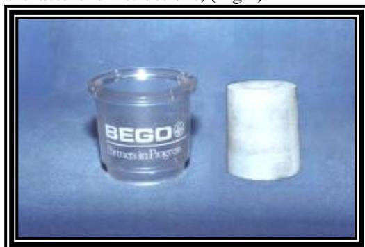
**Figure 2: The muffle of investment disassembled from the plastic ring**
