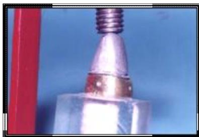
**Figure 3: Close view of preparation margin of the brass die and the gingival margin of the coping**
