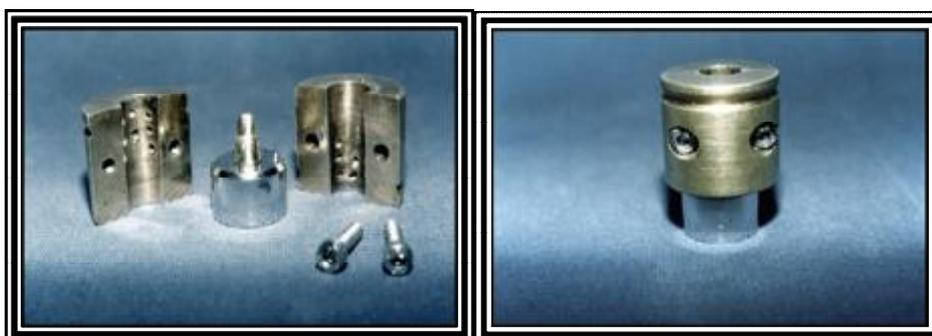
**Figure 1: The split mold framework with the prepared brass die fixed into the mold.**
