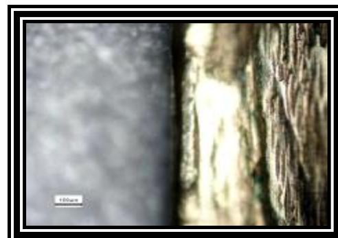
**Figure 13:** Labial marginal gap of coping using the (RA) technique for WYMvest investment
