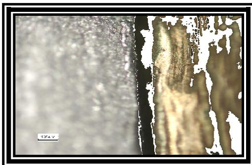
**Figure 9:** Labial marginal gap of coping using the (RLC) technique for BellaStar XL investment.
