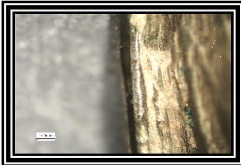
**Figure 8:** Labial marginal gap of coping using the (RC) technique for BellaStar, XL investment. Yellow= brass die. Black= marginal gap, Gray= coping
