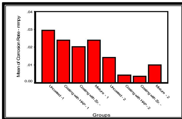
Figure 18: Bar chart plot for mean values of the corrosion rate of Ti-6Al-4V (1) alloy and Cp Ti (2) with different coatings
