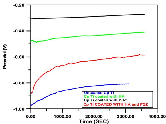
**Figure 12: Open circuit potential for uncoated and coated Cp Ti with different coating materials.**
