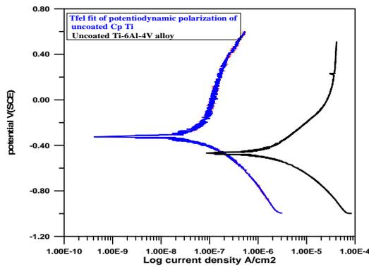
Figure 14: The polarization curves of uncoated Cp Ti and uncoated Ti-6Al-4V alloy.
