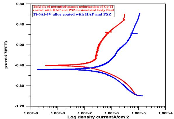
Figure 17: The polarization curves of Cp Ti and Ti-6Al-4V alloy coated with HAP and PSZ.
