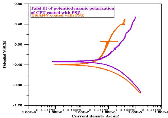
Figure 16: The polarization curves of Cp Ti and Ti-6Al-4V alloy coated with PSZ.
