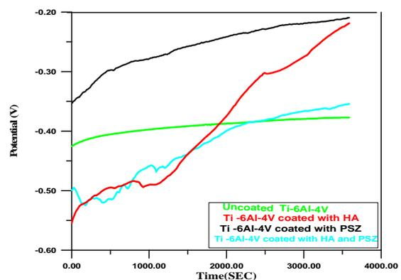
**Figure 13: Open circuit potential for uncoated and coated Ti-6Al-4V alloy with different coating materials**
