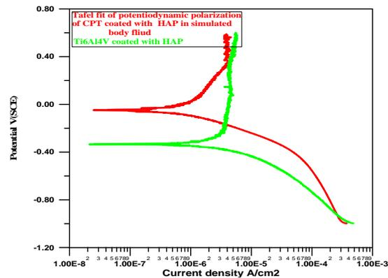
Figure 15: The polarization curves of Cp Ti and Ti-6Al-4V alloy coated with HAP.
