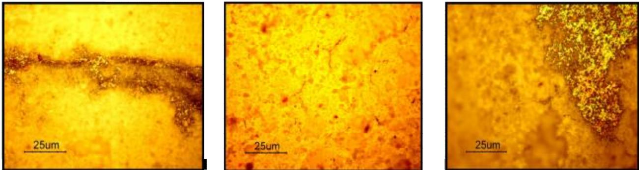
A-Ti-6Al-4V alloy coated with HAP. B-Ti-6Al-4V alloy coated with PSZ. C-Ti-6Al-4V alloy coated with HAP and PSZ.
