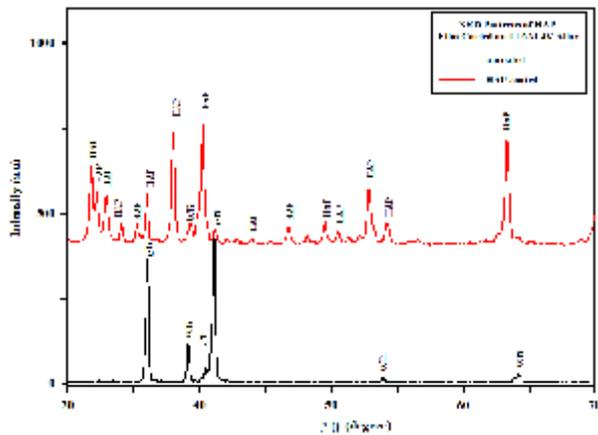
Figure 1: X-ray diffraction patterns of HAP coated Ti-6Al-4V specimens in comparison with uncoated specimen
