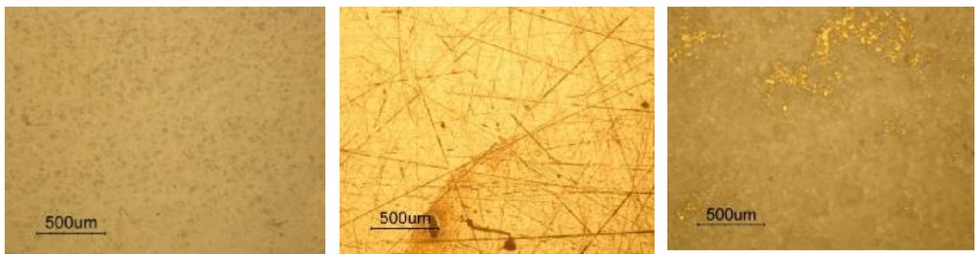
Figure 8: Optical micrograph view of Cp Ti coated with mixture of HAP and PSZ before corrosion
