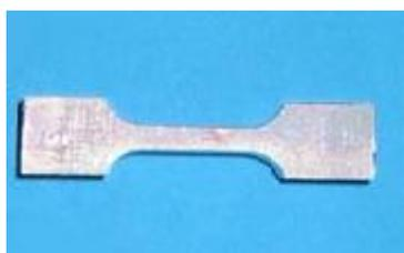
**Figure 1: Metal pattern for tensile strength test**
