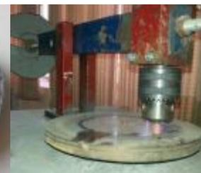
Figure 8: Pin on disk mould with held specimen.
