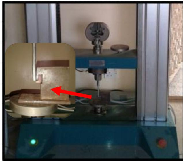
Figure 3: Instron machine with tooth clamp
