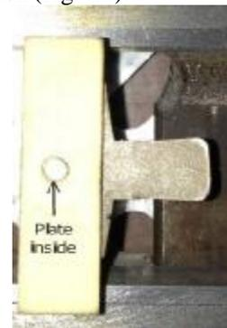
**Fig. 11: The horizontal plate and the insertion guide inside bone block**
