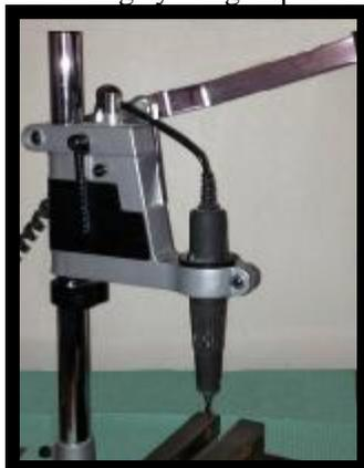
**Fig. 3: Drilling engine stand**
