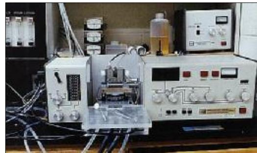
**Figure 4: Flameless atomic absorption spectrophotometer.**
