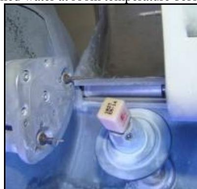
**Figure 4: VITA ENAMIC block inserted in Sirona CEREC in Lab MC XL**
