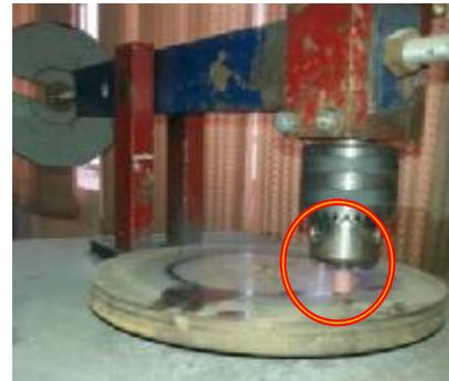
Fig. 3: Pin on disk with the specimen
