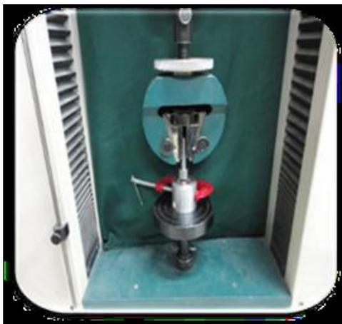
**Figure 4. Chamber of the loading device where load is applied at 90° to the occlusal surface of the tooth.**
