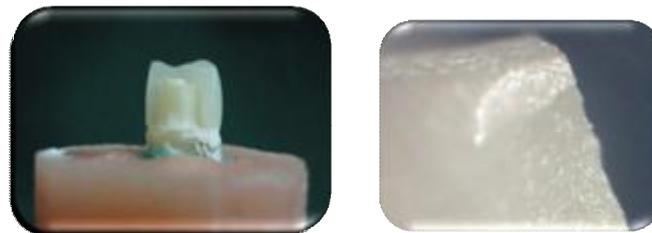
**Figure 6(a). Failure type of a Cergo Kiss crown after fracture test. (b) Optical microscope image of fractured surface of a Cergo Kiss crown (x40 magnification).**
