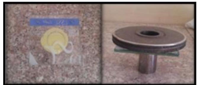
Figure 2: Flat glass plate pressed over the mold
