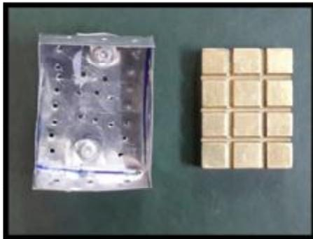
**Figure 6: Brass master model with its aluminum tray**
