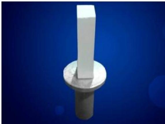
**Figure 1: Parallel sided blank glued on the fitting pin**
