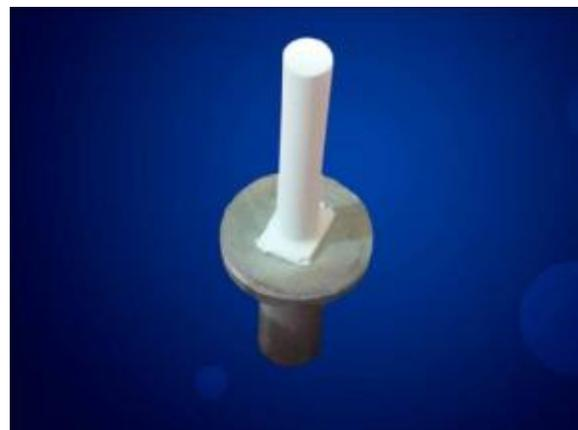
**Figure 3: Cylindrical zirconia blank**
