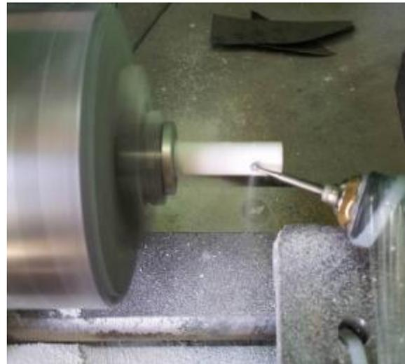
**Figure 2: Milling and cutting the zirconium parallel sided blank**
