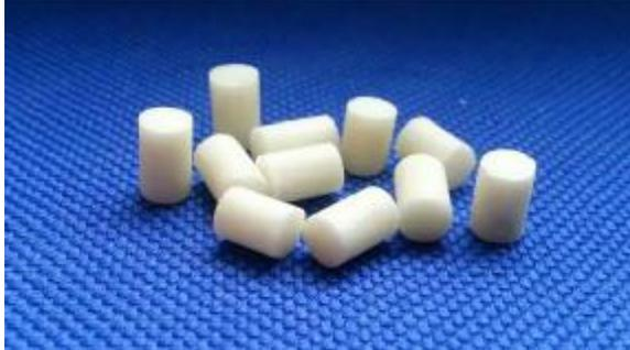
**Figure 5: Final shape and size of the zirconia cylinders**
