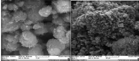
**Figure 3: Nano titania filler under SEM**
