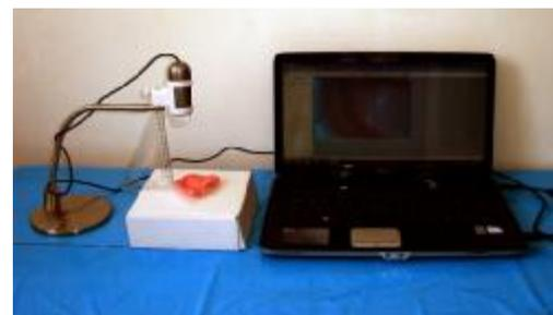
**Fig. 3: Measurement of linear dimensional changes using digital microscope**
