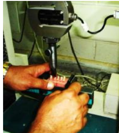
Figure 2: The embedded specimen (teeth in the acrylic block) was secured in the sliding jig
