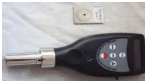
**Figure 1: Compact portable indenter (Shore D hardness tester) with its test block.**
