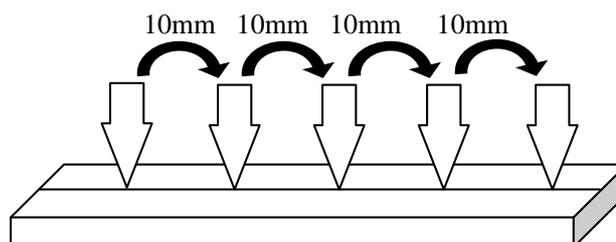
**Figure 2: Schematic diagram of the surface hardness test specimen with five test sites.**
