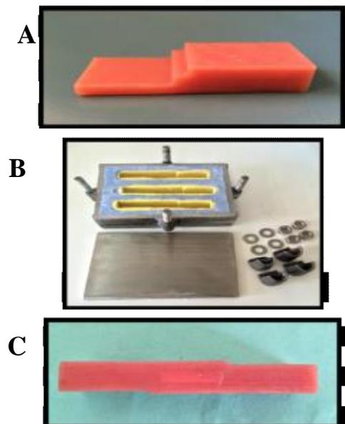
**Figure 2: (A) Acrylic block used in test, (B) Custom-fabricated flask with silicon-stone mould. (C) Shear bond strength test specimen.**
