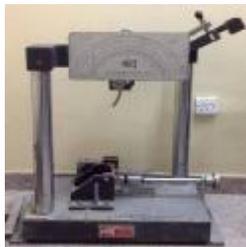
Figure 2: Impact strength testing device
