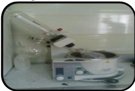
Figure (2): Rotary Evaporator
